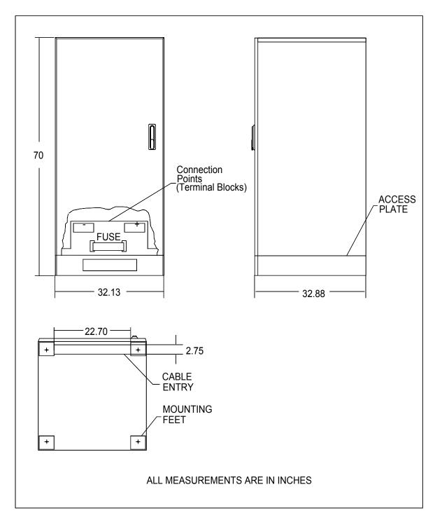
Figure 14 – "C" Battery Cabinet Drawing for 36/50/80kVA Ratings
